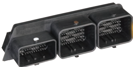
3 pocket CMC Header, series 34763 154-circuits, 48+53+53 Compliant-Pin, Pressfit
